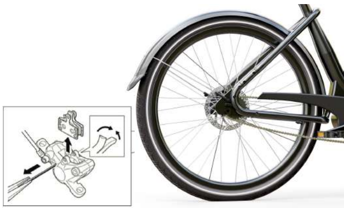
Image 42: Removing the brake pads in order to check them for wear
