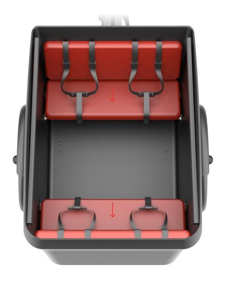
**6-** Place the seat on the brackets, aligned with the Velcro, and push so that the Velcro adheres.
