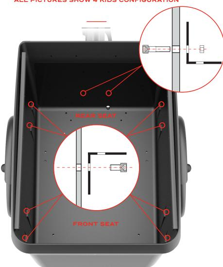
**1-** Mount the brackets on the box, using 2xM4 bolt for each bracket, in the positions shown above. ONLY FOR REAR SEAT: mount a bracket in the middle of the box rear wall, upside down compared to the other brackets (use the bolts and nuts from the steering column).
