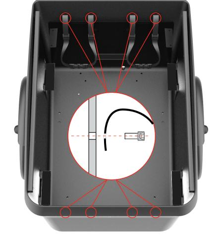
**2-** Connect seat belt shoulder holders to the rear wall on the box with 2xM5 bolt each in the specific threaded holes.
